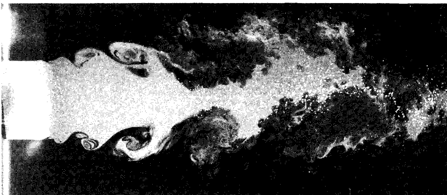
Fig. 2 Unforced particle-laden flow, Re_D = 1.9 \times 10^4 .
